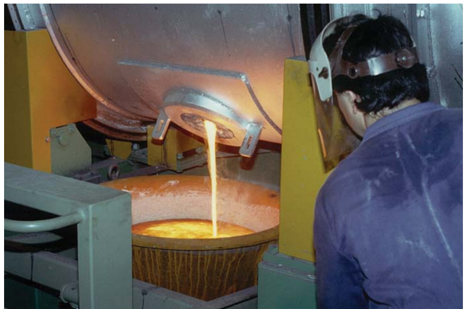
Melted metal from a rotating furnace for the precious metals recovery from ashes.
