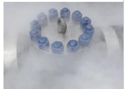
*Valve undergoing a cryogenic test*
