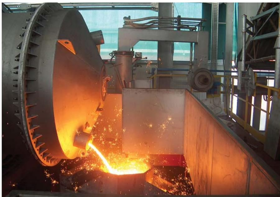
*Oxy-fuel burner in cast iron rotary melting furnace*
