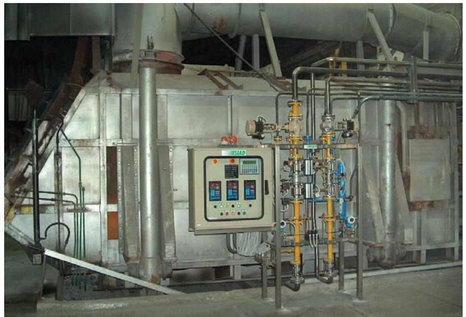
*Oxy-fuel unit for aluminum reverberatory melting furnace*
